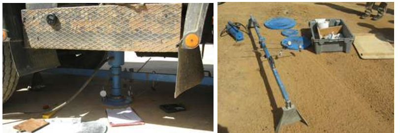
Static Plate Load Test Equipment
